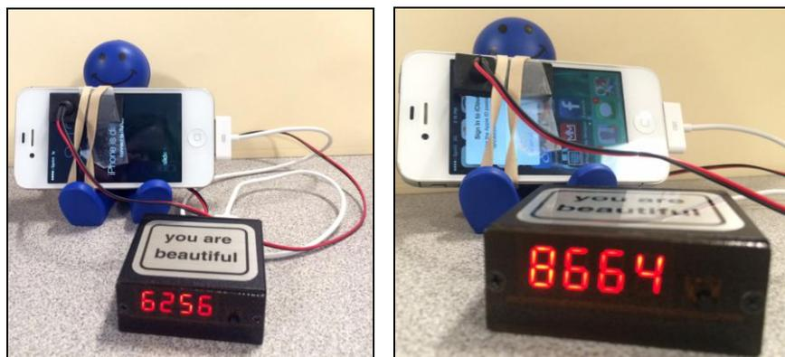
**Battery/Power Tips:** As stated earlier, using an attack that includes all numbers between 0000 and 9999 can take up to 17 hours, and obviously the iOS device’s battery may not last that long. In the image
