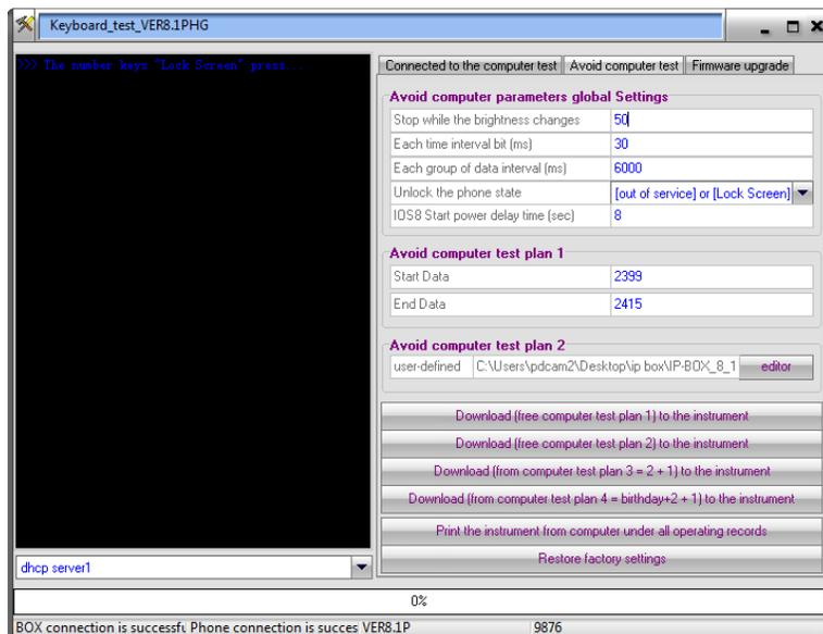
**Avoid computer test plan 1** – by default is set to start at 0000 and end at 9999. Any options can be entered here, including custom ranges as shown above. So you could start at 9999 and end at 0000, or use any range of numbers you wish.
